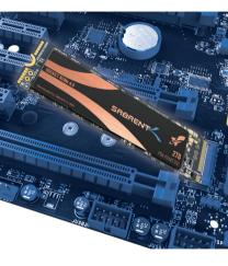
9. Fasten the opposite end of the Sabrent ROCKET NVMe M.2 SSD to the motherboard with the necessary screw or hardware, as is illustrated below.
