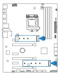
8. Insert the Sabrent ROCKET NVMe M.2 SSD device pin-side first into the M.2 slot as is illustrated below.
