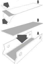
**5.** Place the SSD in the tray on the thermal tape and make sure the groove meant for the screw placed in the back of the drive is flush with the same groove that is in the back of the aluminum tray.
