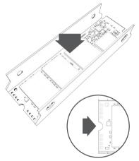
**6.** Attach the tray with the drive to the heatsink ensuring that the side with the uneven coils are on the back, on the side of the groove meant for the screw.
