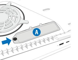
Remove the screw from the expansion slot cover (A) and remove the cover.
