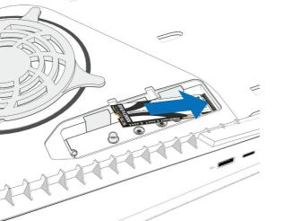
Hold the edge of your M.2 SSD, align it with the notch on the expansion connector, and then, starting from diagonally upward, firmly insert it all the way in.
