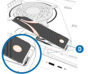
Tilt the SABRENT HEATSINK FOR PS5 CONSOLE expansion slot cover until lip (D) fits into the groove
