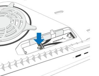
Tilt your M.2 SSD down and fasten it with the screw.
