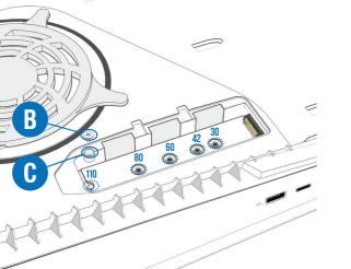
Remove the screw (B) and spacer (C), and adjust the spacer to the size of your M.2 SSD
