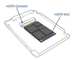
Gently attach your mSATA drive into the housing and connect to the mSATA connector.
