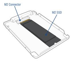
1. Gently attach your m2 ssd drive into the housing and connect to the m2 connector.
