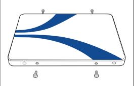
3. Fasten the aluminium case using the 4 screws provided.
