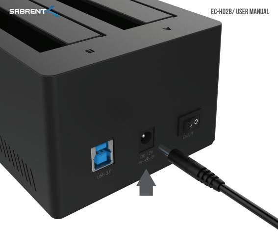
Connect the power adapter to the back of the dock
