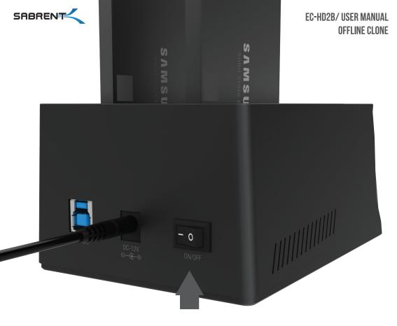
Press the Power Switch to ON
