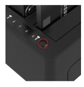
A Blue LED will flash on 25% indicating that the cloning process has begun
