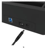
Connect the **USB Cable** to the back of the dock
