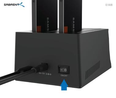
Press the Power Switch to ON
