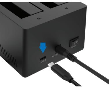
Connect the USB cable to the back of the dock
