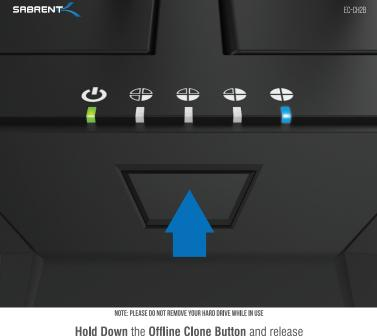
Hold Down the Offline Clone Button and release when you see a Blue LED illuminate in the Status LED Indicator
