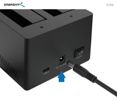
Connect the power adapter to the back of the dock
