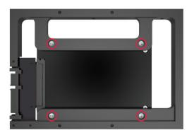
3 - Insert the Sabrent converter with the mounted hard drive into the computer.
