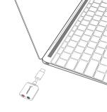
Plug USB Audio Sound Adapter into Type-C port of computer or laptop -- make sure "SABRENT" text on USB Audio Sound Adapter is face up.
